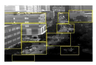
After setting the ROI area, the temperature of each ROI and the isothermal color, the setting values are transmitted to the relevant camera.
