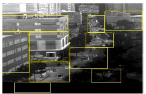
After setting the ROI area, the temperature of each ROI and the isothermal color, the setting values are transmitted to the relevant camera.
